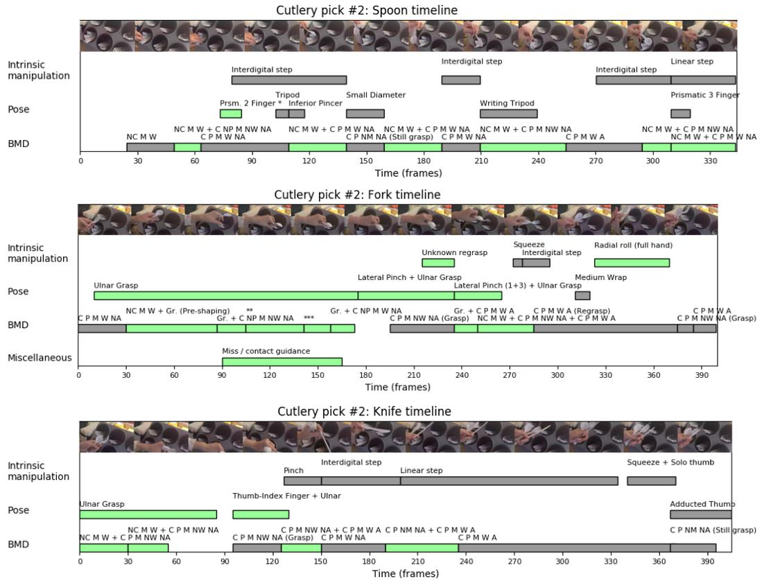
**Figure 4.5:** Timelines for cutlery pick #2. \*This grasp is capable of sliding the spoon out, but part of the spoon is supported by the environment, so this grasp is an environment-aided prehensile grasp. \*\*NC M W + C P M W NA + C NP M W A (different fingers holding, pre-shaping, and manipulating). \*\*\*NC M W + C P M W NA + C NP M W A (same as previous but with full-arm motion)
