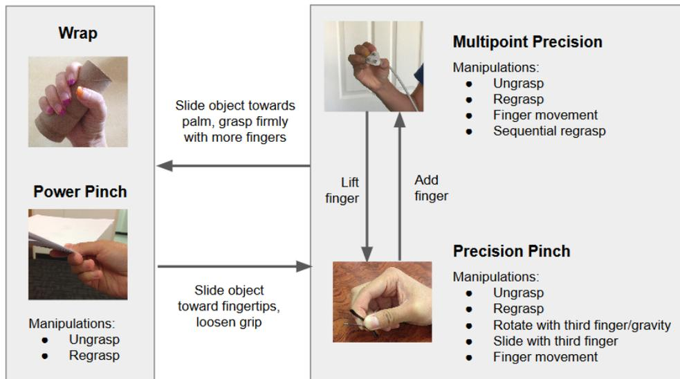
Figure 5.11: Summary of grasp types, types of manipulation possible at each, and general patterns of transitioning between them. Not shown: the non-prehensile point contact.
