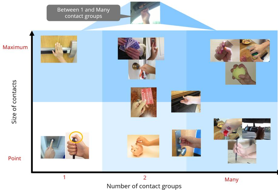
**Figure 5.12:** Axes underlying our pose classification: number of contact groups and size of contacts. Some grasps are in-between types.
