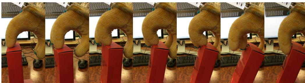
**Figure 8.10:** Hardware results for motion 3. Screenshots 1-3: initial position and motion with front fingers. Screenshots 4-5: motion with back fingers. Screenshots 6-7: front finger reset and first frame of motion.
