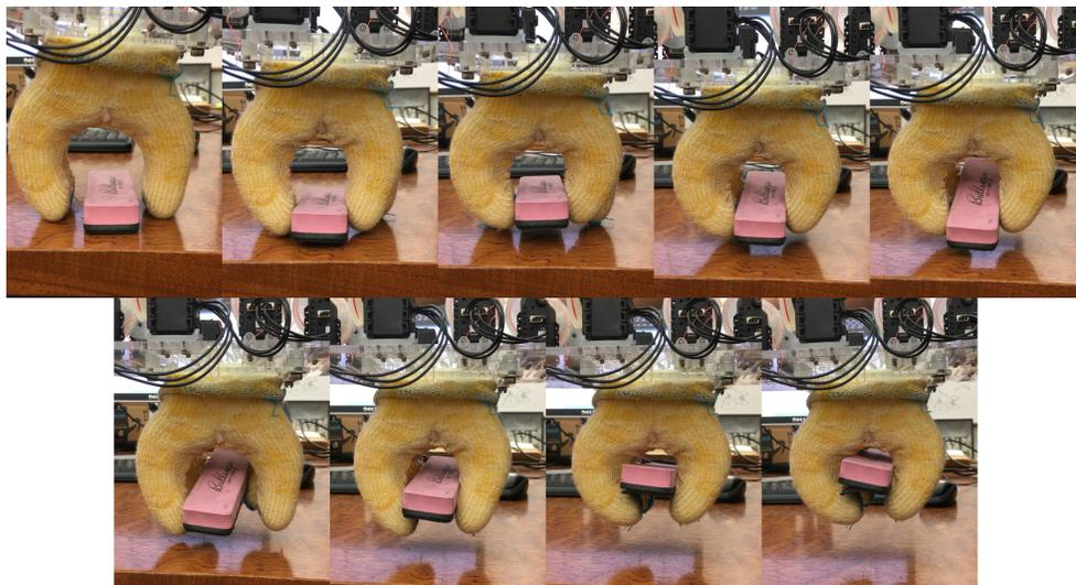
**Figure 8.9:** Hardware results for motion 2. Screenshot 1: initial position. Screenshots 2-3: motions with front fingers. Screenshots 4-5: motions with back fingers. Screenshots 6-8: resetting front fingers and repeating motion. Screenshot 9: final power grasp.
