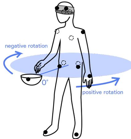
**Figure 6.10:** Motion capture setup for Experiment 2. The black and dotted circles represent the placement of 16 reflective markers on the front and back of the participant. The direction of the bowl is defined as zero degrees (the direction of the goal is  $\pm 180^\circ$ ) and counterclockwise rotations are positive angles.
