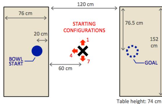
**Figure 6.9:** Experiment 2 setup with only one starting location (with three facing directions).
